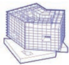
Exterior Wood Grid System
